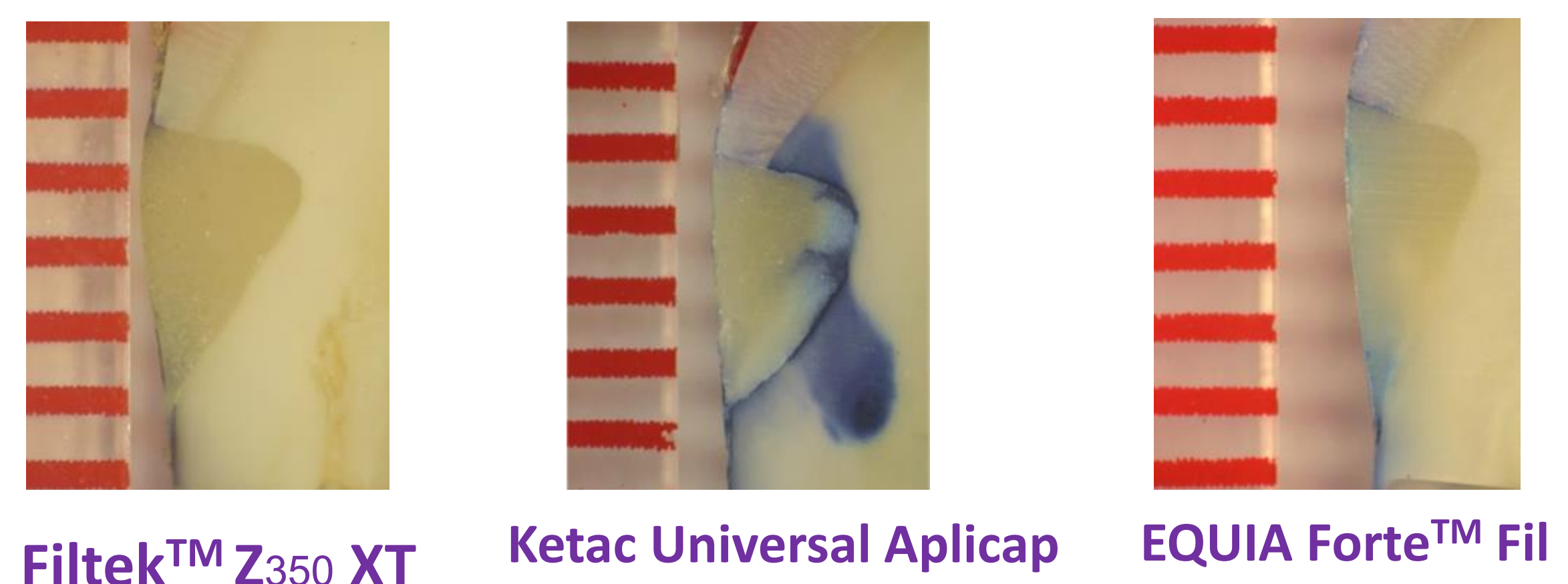
Picture 1 the sample pictures of microleakage took from stereoscopic microscope
