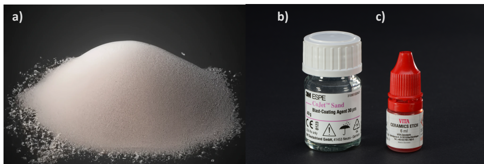
Figure 1. Investigated materials for mechanical pretreatment. a) Alumina sand 35 µm (Hasenfratz, Germany) for grit blasting. b) CoJet Sand (3M, Germany) for tribochemical silica coating. c) Hydrofluoric acid (VITA Ceramic Etch, VITA, Germany) for etching.
